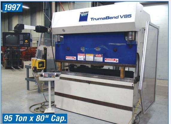
1997 **TRUMPF** V85 6 axis CNC press brake with DELEM DA-65 CNC Control, 4 axis back gauge, CNC crowning, hydraulic clamping, safety lights, s/n 883215
