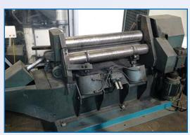
ELAM 3' X 1/4" 4 ROLL INITIAL PINCH ROLLS, 5" DIA ROLLS
